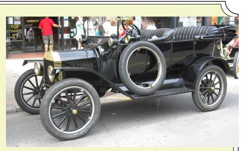
two fastened to its rear. A hand-operated air pump and a rubber tube patching kit were also an essential part of traveling. For a weekend of touring those four spare tires might not have been enough, and it would be necessary to dismantle a tire, remove the inner tube, locate and patch the puncture.
