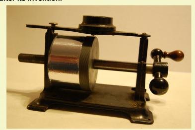
The talking machine was invented in 1877 by Thomas Edison in his laboratory at Menlo Park, New Jersev. Aware that sound can be produced by vibrations, he made a rough sketch of a vibration recording reproducing device of which he had conceived and asked his machine shop foreman to have it built. The next day he was presented with the result. a creation almost identical with the replica on display here.
